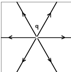
The technique remains the same as above. The direction of the electric field is along the field lines, and the comparative strength is given by the density of lines. (When the density of field lines doubles, the field strength does not necessarily double also, because you are not seeing all the lines. All you can say is that the field gets stronger.)
